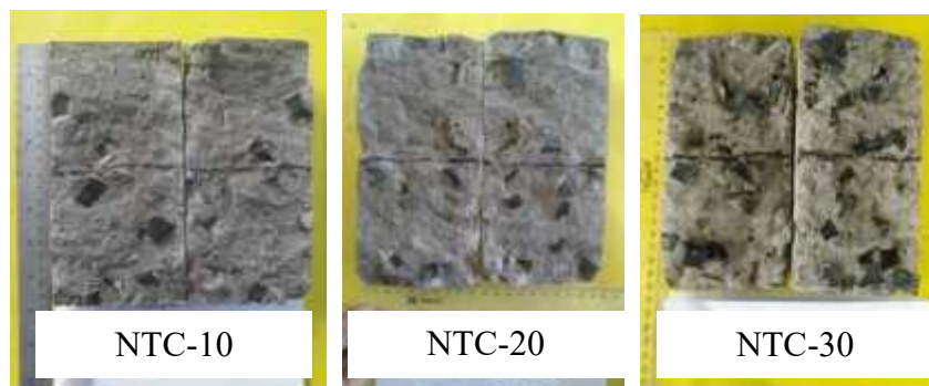
Figure 3. Tire chip detached from concrete paste.
